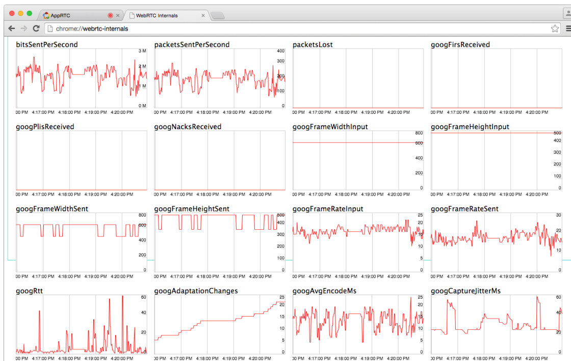
Figure 7: Real-time Plots generated from WebRTC getStats()
