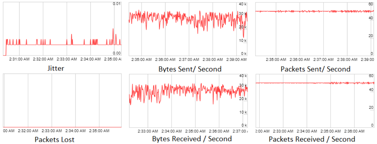
Figure 23: Packets and bytes sent and received (per second), jitter, and packet loss for audio data
