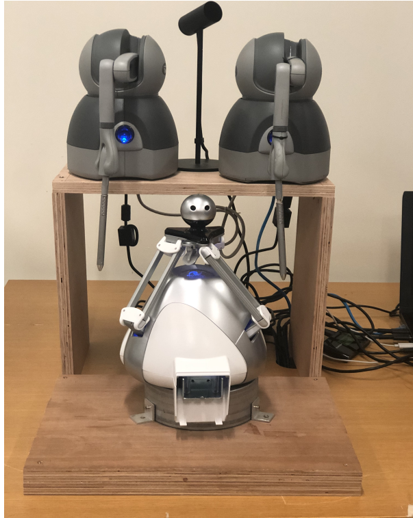
Figure 10: Haptodont Front View: Two Geomagic Touch haptic devices on top with Oculus Rift Camera , and Novint Falcon Finger Support on the Base.
